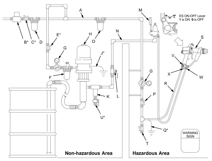
The air supply to the gun must be electrically interlocked with the ventilators to prevent the power supply from operating without ventilating fans on.
